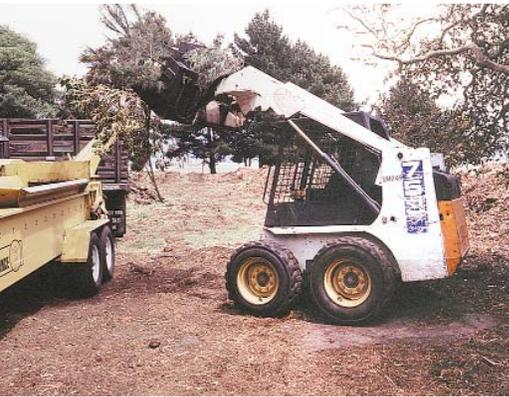
At first, Rubicon staff tried to load all the plant trimmings into the chipper by hand. It quickly became apparent that the staff would not be able to keep up with the grinder. A Bobcat with a grapple bucket is now used to load the machine more efficiently.
